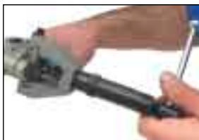
Step4 Turn T-Bar to create the flare.
