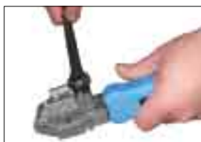
Step2 Tighten the clamping nut.
