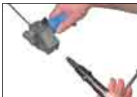
Step3 Insert the punch and ram.
