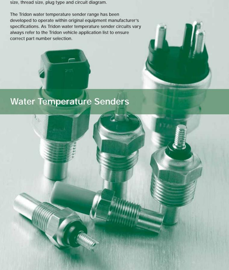
The water temperature sender is used to measure the integrity of the engine cooling system. Located on the engine side of the thermostat in the cooling system, the water temperature sender responds to changes in engine coolant temperature modifying the signal from engine temperature instrumentation. This modified signal is used to determine the engine coolant temperature via water temperature light or gauge.
